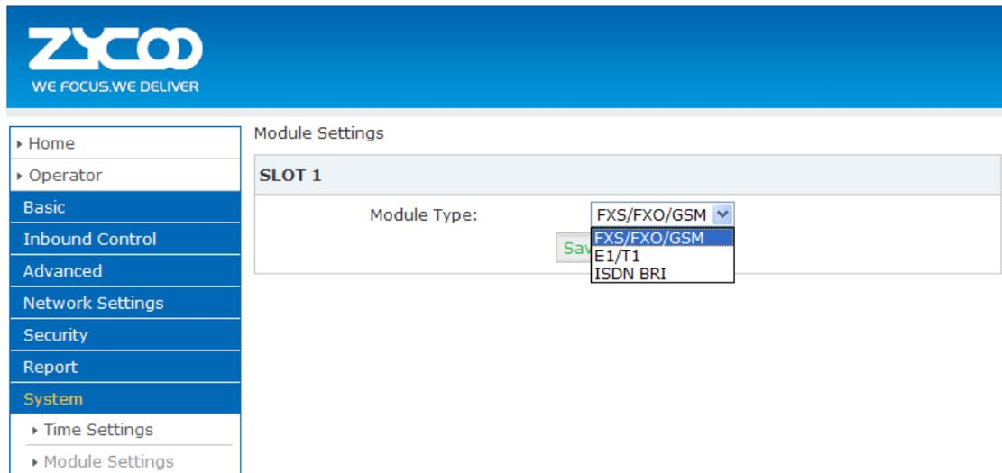
Select the module type, which is same as your installed module. Click **【Save】** and finish the module configuration. (Module installed in SLOT 2 can be identified automatically, no need to configure it.)
